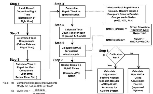
Figure 2: Approach to Estimating MCR for Aircraft
