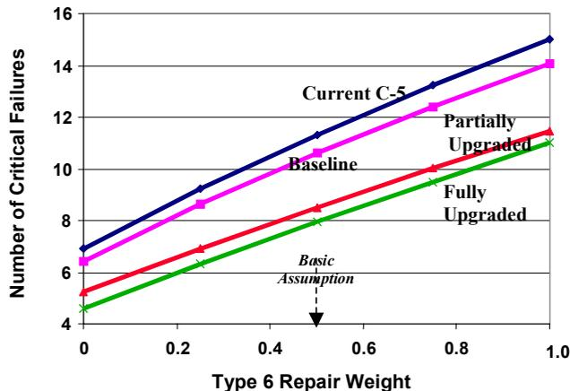
Figure 5: Type 6 Repair Weight vs. Critical Failures
