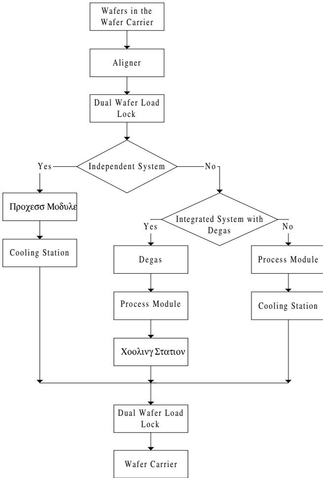
Figure 4: The System Process Flow
