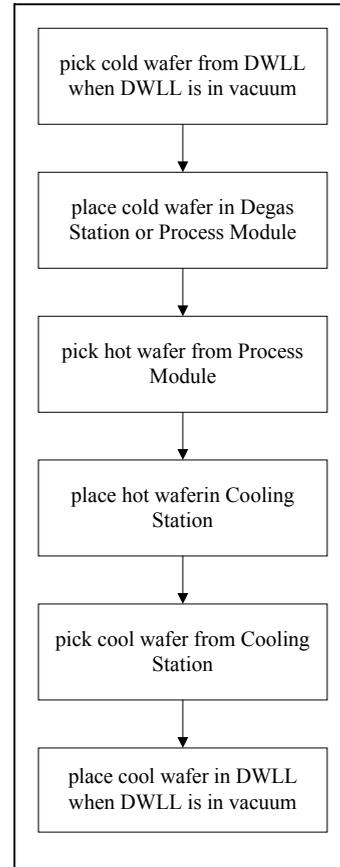
Figure 3: Vacuum Robot Tasks
