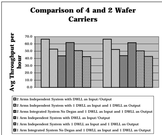
Figure 6: Comparison of Throughput of 4 and 2 Wafer Carrier Systems
