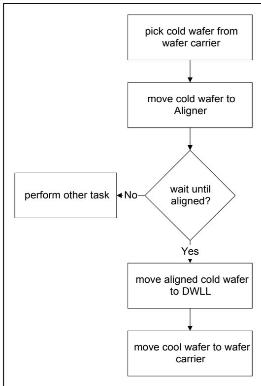
Figure 2: Atmospheric Robot Tasks
