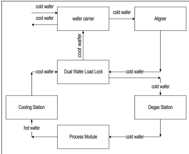
Figure 1: Flow of Wafers through the System
