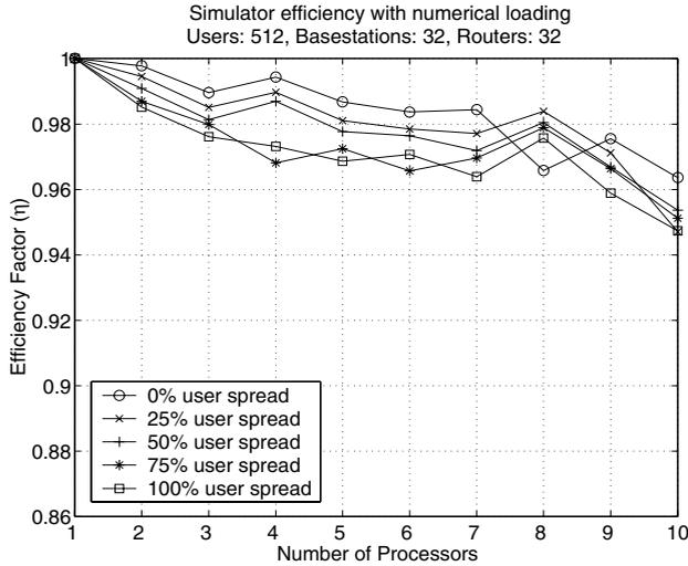
Figure 7: Simulation Efficiency as a Function of Number of Processors. 512 Users, Numerical Loading Enabled
