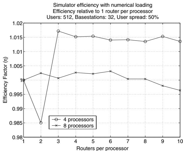
Figure 10: Simulation Efficiency as a Function of Routers per Processor. 512 users, Numerical Loading Enabled
