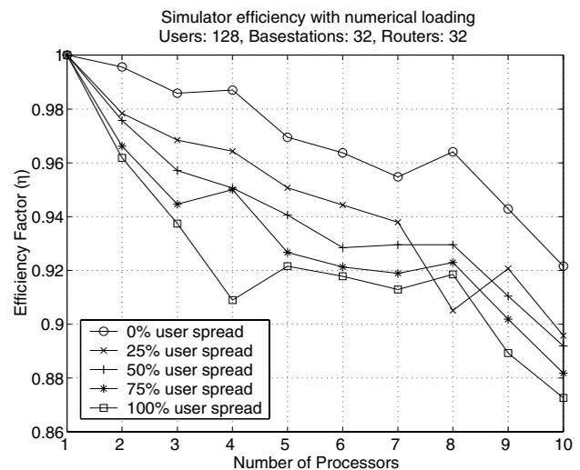
Figure 6: Simulation Efficiency as a Function of Number of Processors. 128 Users, Numerical Loading Enabled
