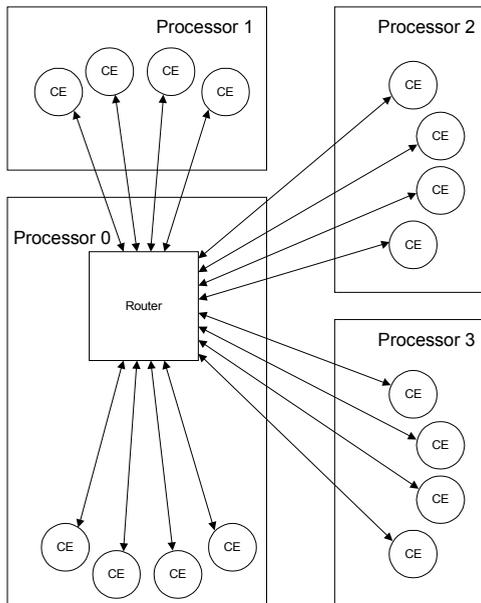
Figure 1: Single Router System
