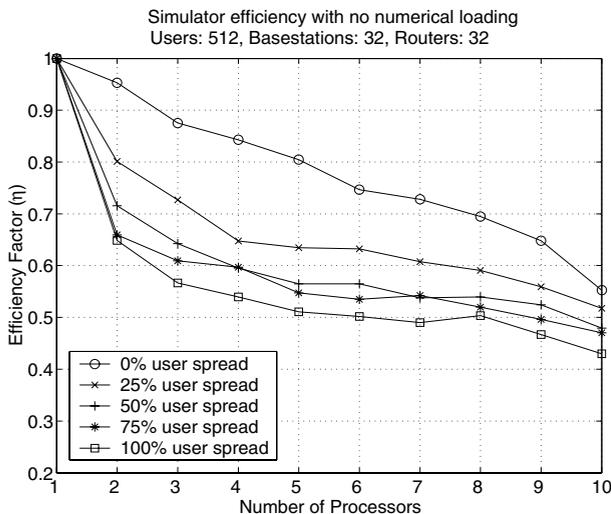
Figure 5: Simulation Efficiency as a Function of Number of Processors. 512 Users, Numerical Loading Disabled
