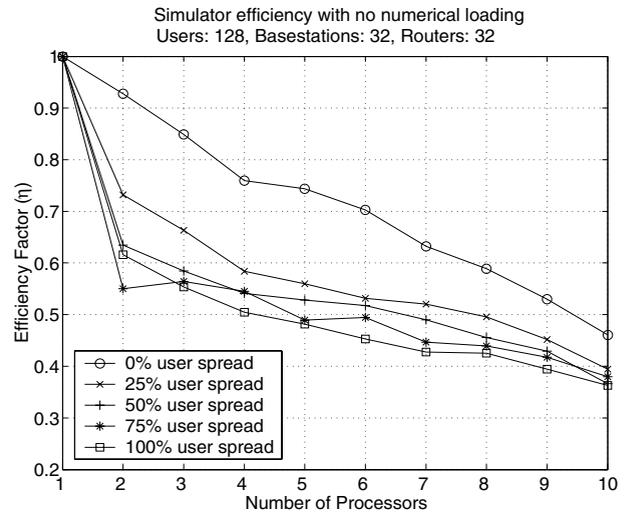
Figure 4: Simulation Efficiency as a Function of Number of Processors. 128 Users, Numerical Loading Disabled
