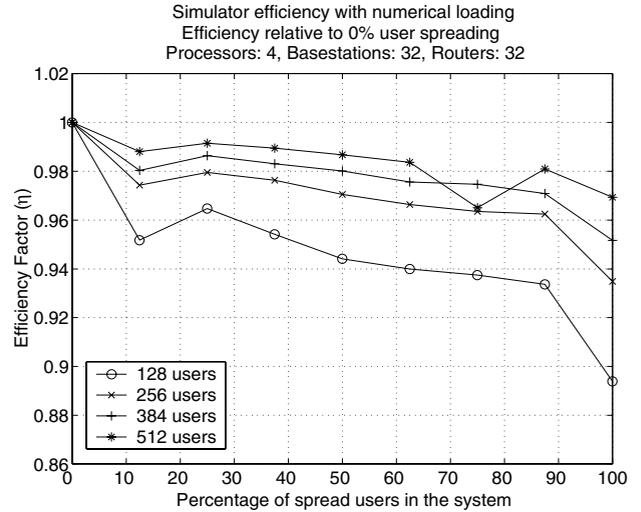
Figure 8: Simulation Efficiency as a Function of User Spread. 4 Processors, Numerical Loading Enabled
