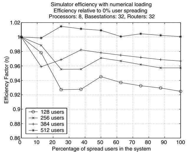
Figure 9: Simulation Efficiency as a Function of User Spread. 8 Processors, Numerical Loading Enabled
