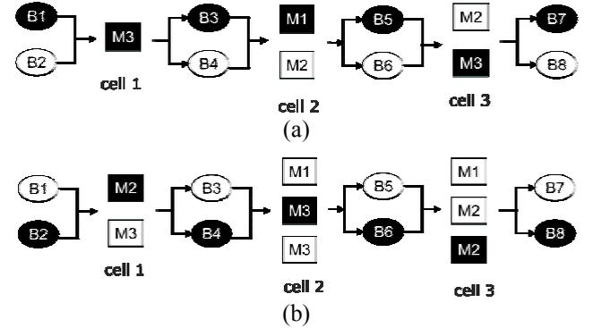
Figure 2: Example 2-Period Capacity Allocation of a 3-Cell Production System: (a) Period 1 and (b) Period 2
