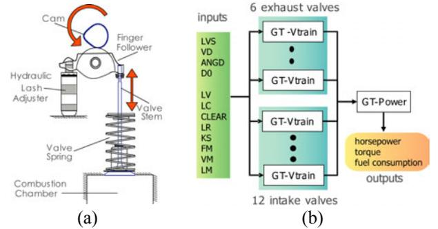
Figure 5: (a) Valvetrain (Kazancioglu *et al.* 2003, Kazancioglu 2004); (b) Integrated Valvetrain-Engine Simulation
