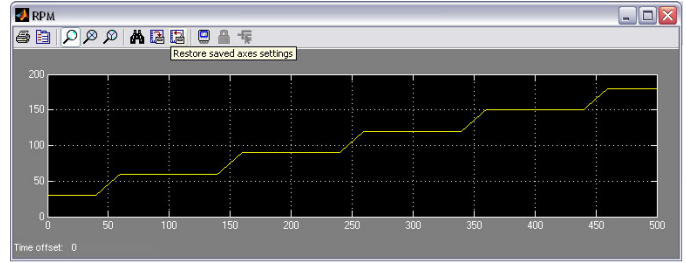
Figure 10: SimMechanics Output for Sphere at 60% Fill Level. [rotational speed (RPM) vs. time (s)]
