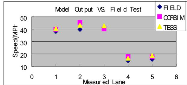
Figure 9: Model and Field Test Speed output at Peak Time in JSKX.
