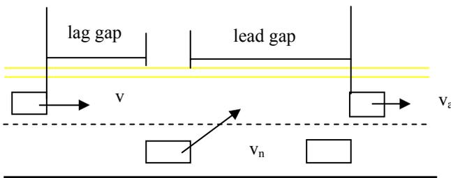
Figure 4: Lead Gap and Lag Gap
