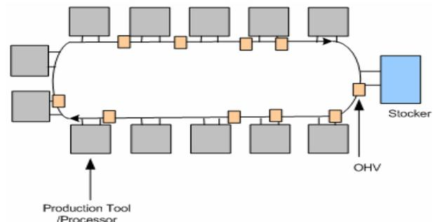
Figure 2: Unidirectional Closed-Loop Overhead Transport System
