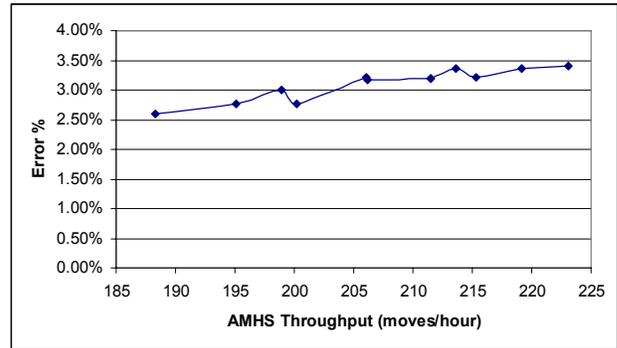
Figure 7: Comparison of Queuing and Simulation Model Throughput Estimates at Different Release Rates.
