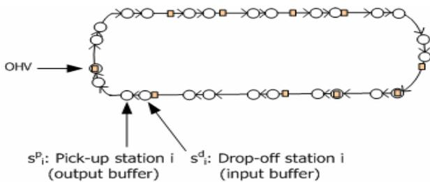
Figure 3: Network Representation of the Closed Loop AMHS
