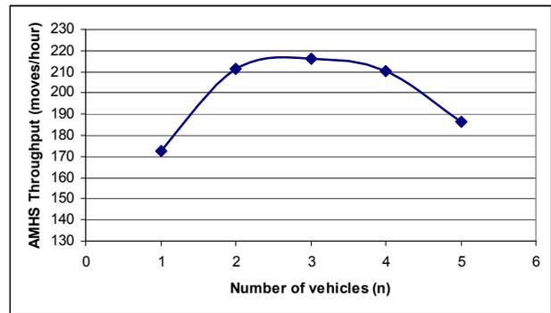
Figure 8: Impact of Increasing AMHS Fleet Size on Throughput.
