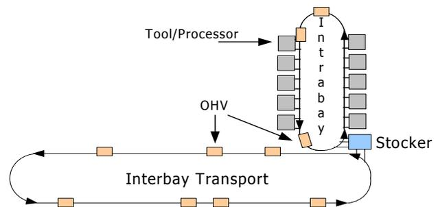
Figure 1: Closed-Loop Unidirectional Interbay and Intrabay AMHSs
