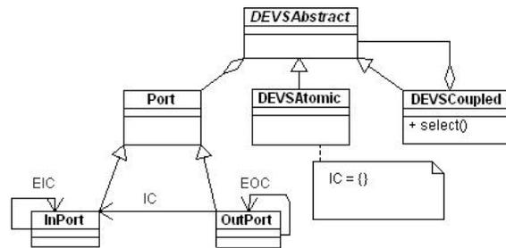
Figure 3: Class diagram of a DEVS coupled model based on the composite pattern.
