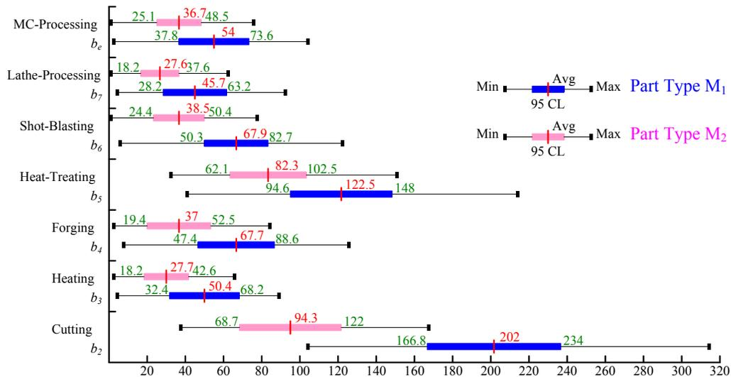
Figure 7: WIP inventory level of simulation results from the AS-IS model.
