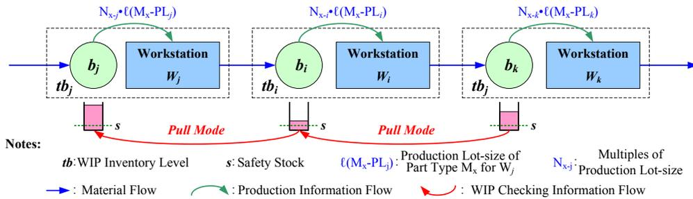
Figure 4: The logic of the Pull production mode based on an inventory level rule.
