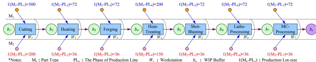
Figure 3: Production line logical structure for part types  $M_1$  and  $M_2$ .
