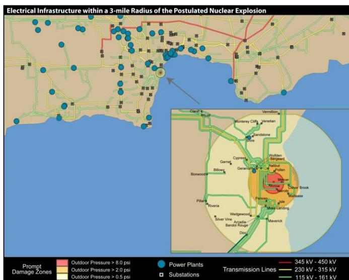
Figure 1: Electric infrastructure serving Any City and 3-mile radius of the postulated nuclear-explosion damage zone.
