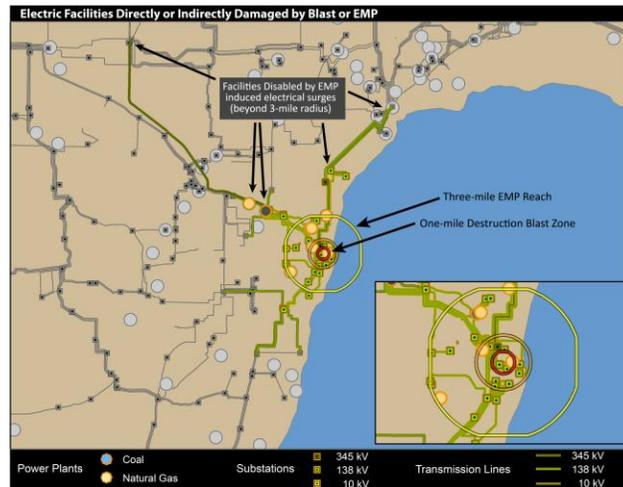
Figure 3: Electric facilities (Categories 1 and 2) instantly affected by the blast and EMP.
