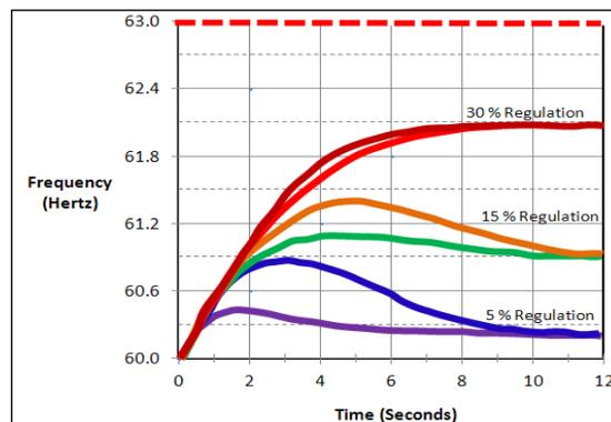
Figure 2: Frequency response to a sudden 10% loss of load.
