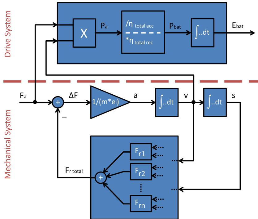
Figure 1: Load model structure.
