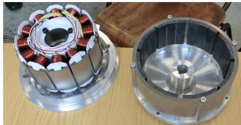
Figure 11: Outer rotor motor with concentrated windings and ferrite magnets (94 % Efficiency).
