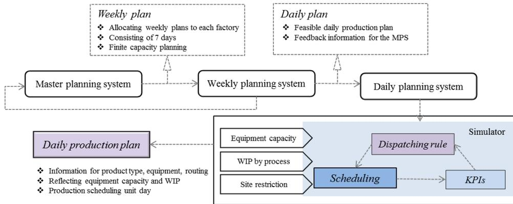
Figure 2: Simulation-based APS.
