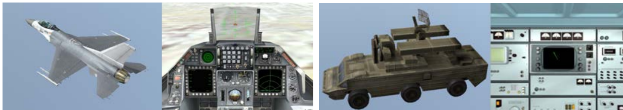
Figure 3: SIMbox training environment for F-16 fighter and SA-8 anti-air missile launcher. This environment can be integrated with an actual cockpit (with joysticks, etc.) to provide more realism.
