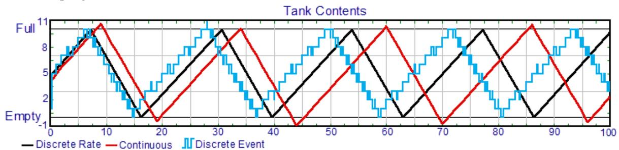
Figure 1: Discrete rate, continuous, and discrete event simulation compared
