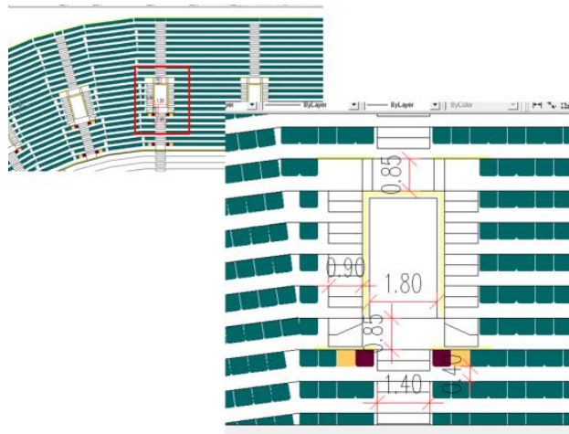
Figure 6: Dimension details of the stadium.
