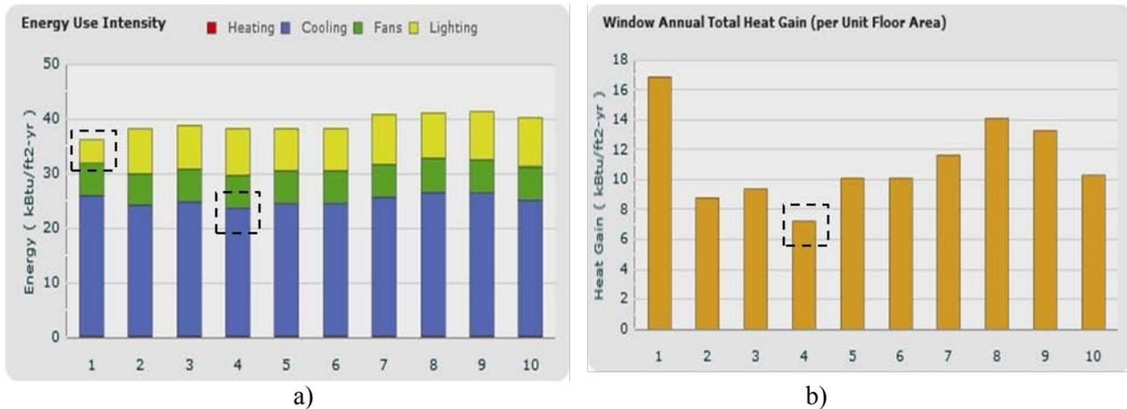
Figure 4: Analysis of second set of window-shading assemblies a) Energy consumption b) Annual heat gains through glazing.
