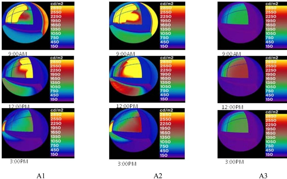
Figure 10: Rendered images from Radiance showing luminance ranges for the selected assemblies (A1, A2, A3) during different times of a summer day (June 21<sup>st</sup>).
