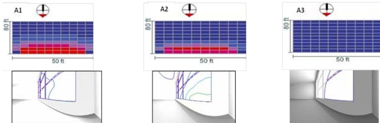
Figure 9: Daylight analysis- Top: Daylight illuminance maps; Bottom: Perspective view illuminance contour lines.
