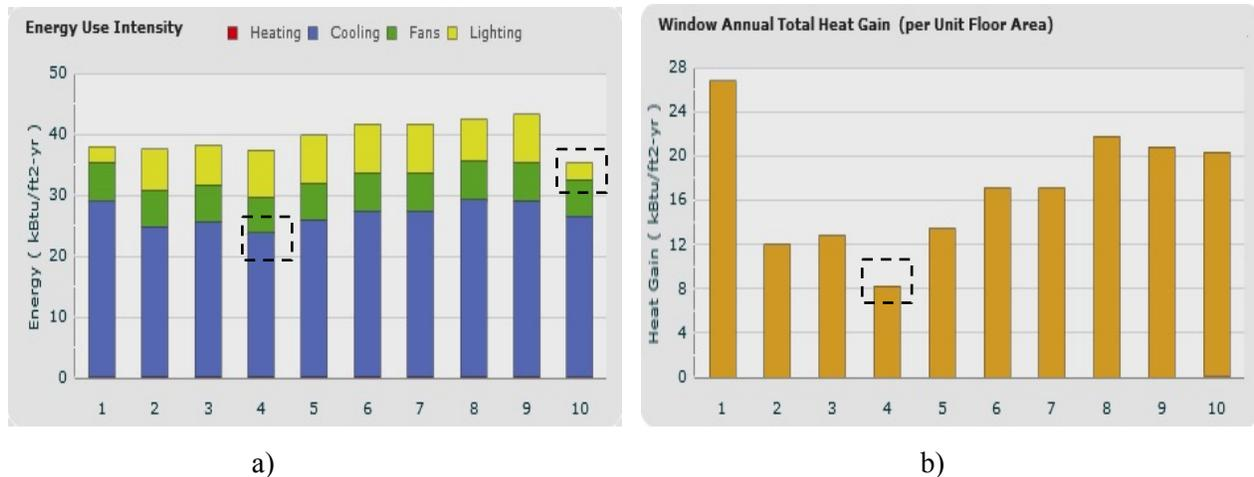
Figure 3: Analysis of the first set of window-shading assemblies a) Energy consumption b) Annual heat gains through glazing. Horizontal axis: 1-no sunshade; 2-External venetian blind 45°; 3-External venetian blind 90°; 4-External roller shade; 5-External screen; 6-Between glass venetian blind; 7-Between glass roller shade; 8-Internal venetian blind; 9-Internal roller shade; 10- Overhangs
