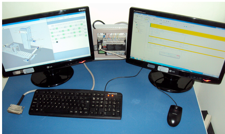
Figure 4: Test environment of the control system with the simulation model. Computer on the left: simulation model in Ururau; computer on the right: Ladder diagram of the control system.
