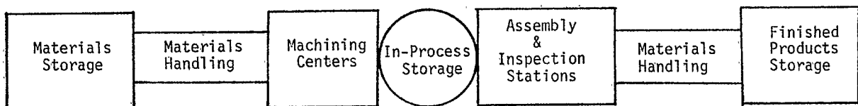
Figure 1: Block diagram of the functional components in a simple manufacturing system.
