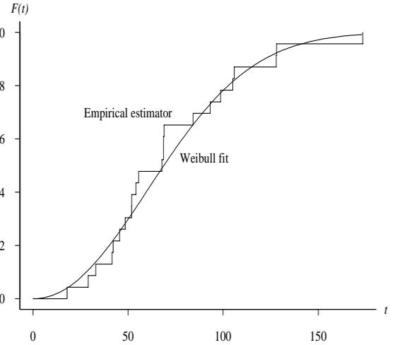
Figure 4: Empirical and Fitted Cumulative Distribution Functions for the Service Times
