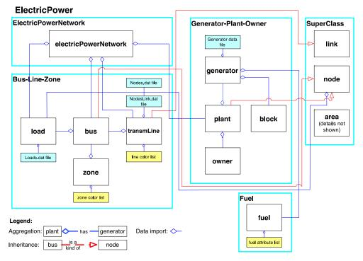
Figure 2: UML class diagram for electric power grid.
