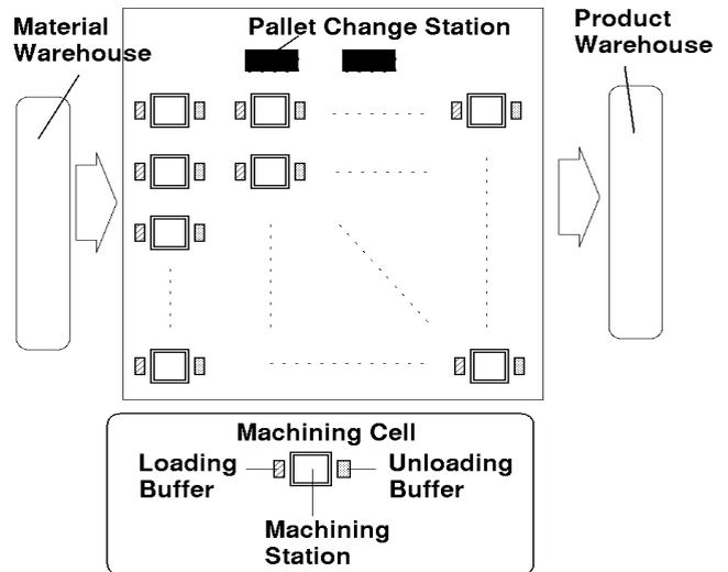
Figure 1: System Configuration of Square Array MCs
