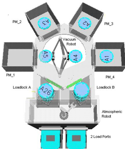
Figure 1: Six-sided Cluster Tool Configuration
