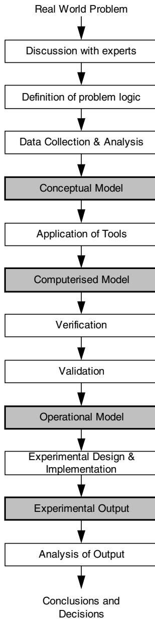
Figure 1: A Simulation Modelling Process
