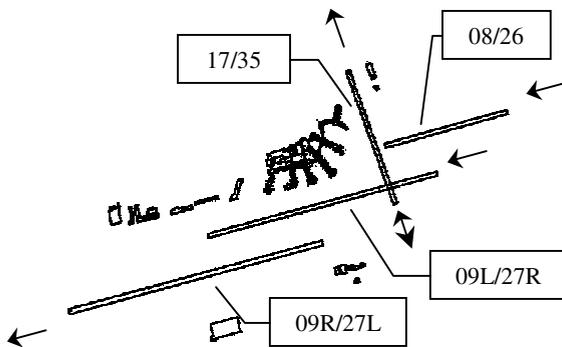
Figure 4: Current West-VFR Operations at PHL
