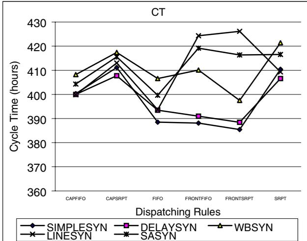
Figure 8: CT under CONWIP Input Rule
