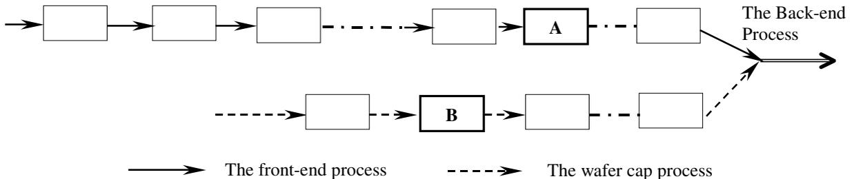
Figure 4: Schematic Representation of WBSYN Rule with the Virtual Flow of the Front-end and the Wafer Cap Process
