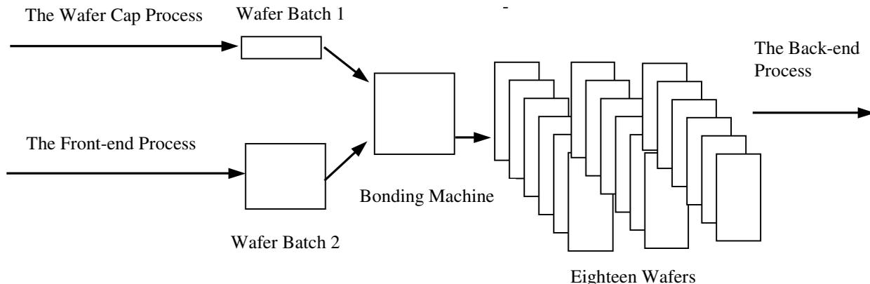
Figure 1: Schematic View of the Whole MEMS Process
