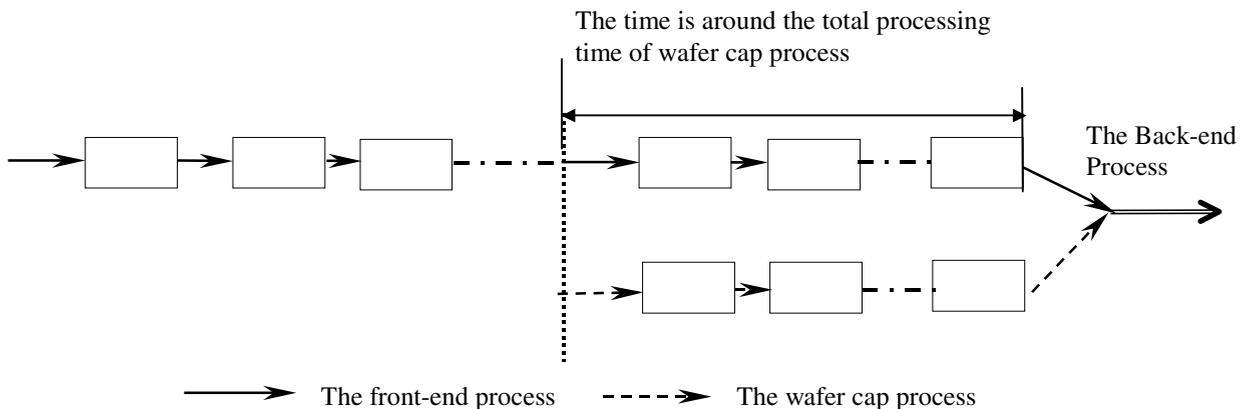
Figure 5: Schematic Representation of SASYN Rule with the Virtual Flow of the Front-end and the Wafer Cap Process
