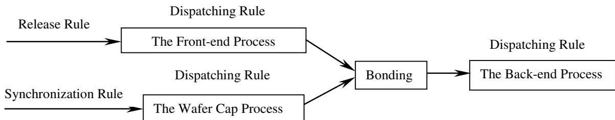
Figure 2: Schematic of the MEMS Fabrication Process with Three Types of Rules
