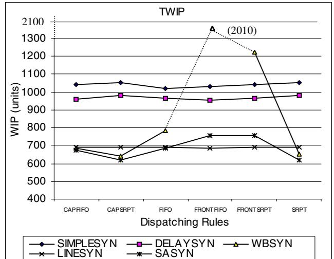
Figure 13: TWIP under CONWIP Input Rule
