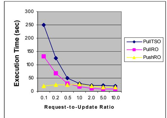
Figure 8: Execution Time vs Request-to-Update Interval Ratio (Lookahead=100)
