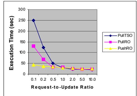
Figure 9: Execution Time vs Request-to-Update Interval Ratio (Lookahead=1000)
