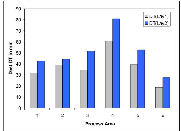
Figure 7: Destination Delivery Time  $DT_{dest}$  for each Process Area - Layout 1 vs. Layout 2
