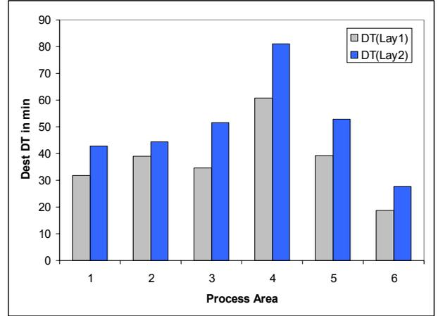
Figure 7: Destination Delivery Time  $DT_{dest}$  for each Process Area - Layout 1 vs. Layout 2
