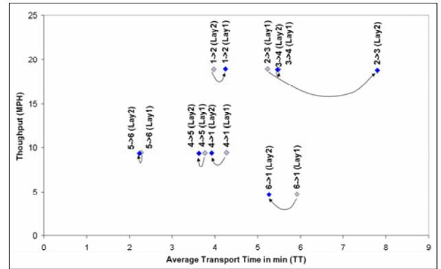
Figure 8: Process Area to Process Area Transportation Time  $TT(src,dest)$  - Layout 1 vs. Layout 2
