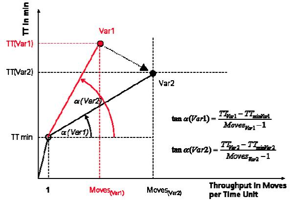
Figure 3: Comparison of a Node-to-Node Connection of two Layout Variants with the TT/Moves Ratio
