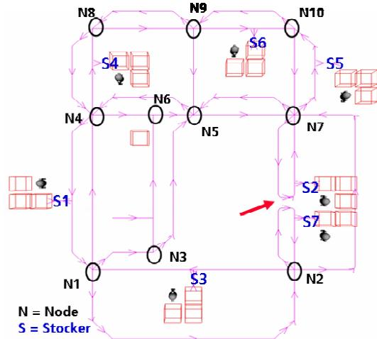
Figure 5: AMHS Layout 2 with Separated PPorts S2 and S7
