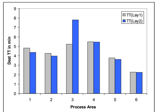
Figure 9: Destination Transportation Time  $TT_{dest}$  for each Process Area (Layout 1 vs. Layout 2)
