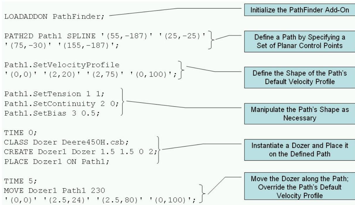
Figure 4: Moving Simulation Objects on Defined Motion Paths
