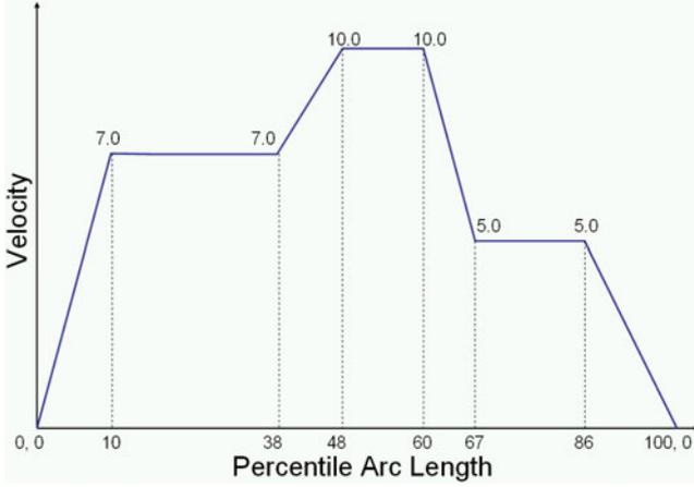
Figure 2: Definition of Velocity Profile Shape
