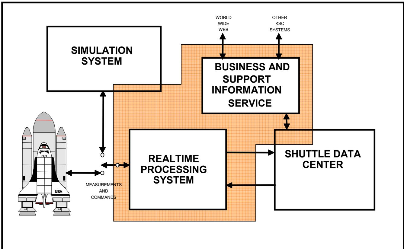
Figure 4: Launch and Simulation System Architecture (from SGOS Developers 2003)
