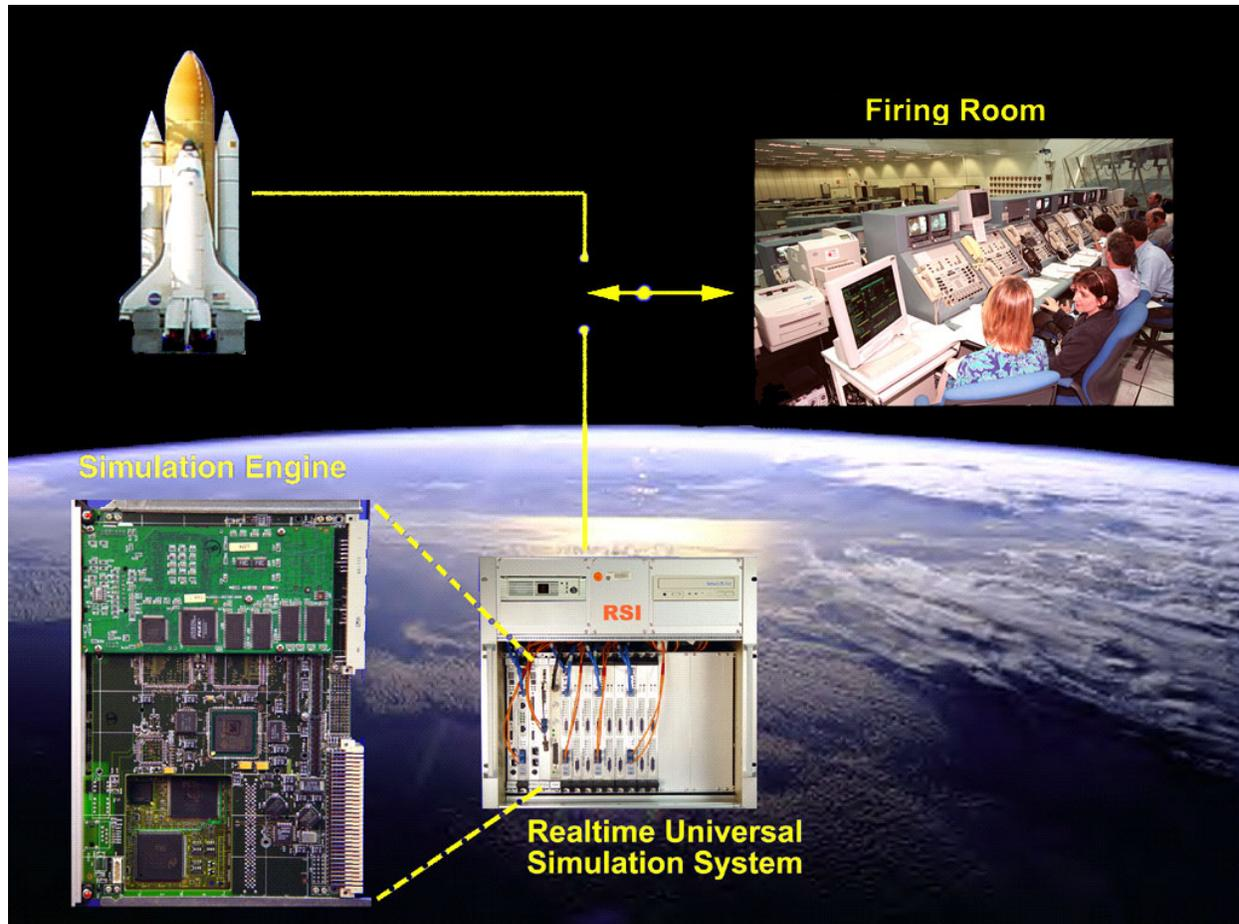
Figure 5: Real-time Universal Simulation System Simulates the Vehicle and GSE (modified from SGOS Developers 2003)
