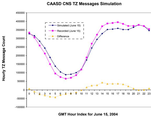
Figure 5: A Simulated TZ Message Profile Over Time
