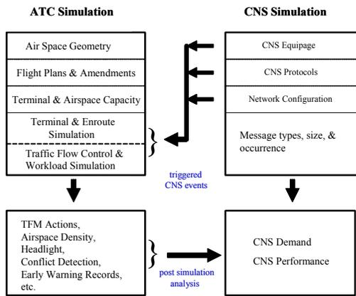
Figure 1: Coupling ATC Simulation with CNS Events
