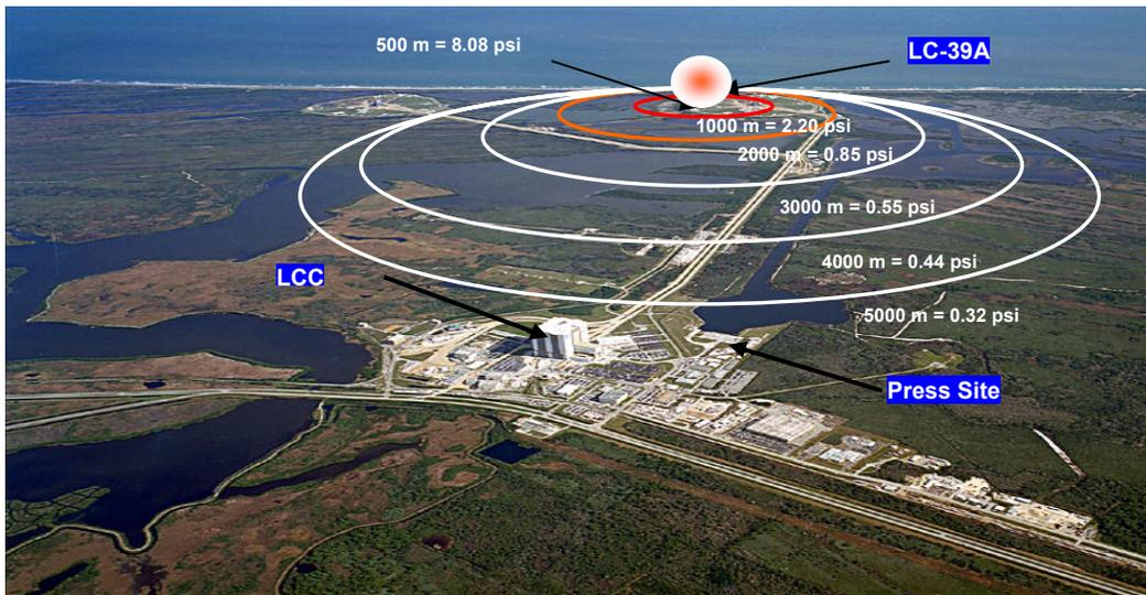
Figure 4: Blast Wave Overpressure Resulting from a Simulated Explosion Ten Seconds after Liftoff
