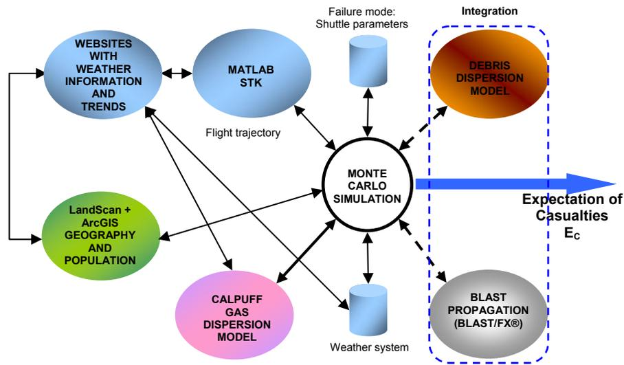
Figure 1: Individual Launch Support Components Integrated into a Virtual Range System Architecture
