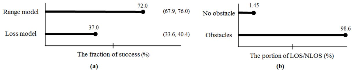
Figure 5: Experimental results: (a) fraction of successful communication on a range model and the proposed loss model (numbers in parenthesis indicate 95% confidence interval) and (b) portion of LOS and NLOS condition.
