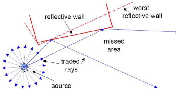
Figure 3: A description of ray tracing method (Bohacek et al. 2004).
