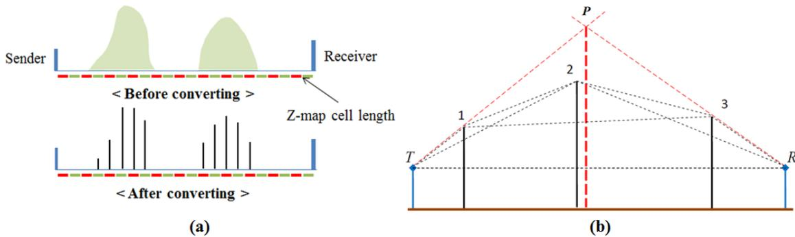
Figure 4: (a) Converting two obstacles into several knife edges in the height-map model of Figure 2 and (b) geometry for the Bullington method (Akkash 2009).
