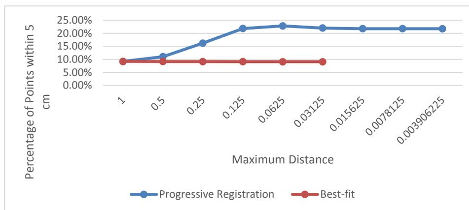
Figure 3 The change of the “5 cm fit percentage” along a progressive registration process, and the corresponding results for using ICP algorithm adopting a single “maximum distance” value (the curve of “best fit,” the unit of “maximum distance” is meter)
