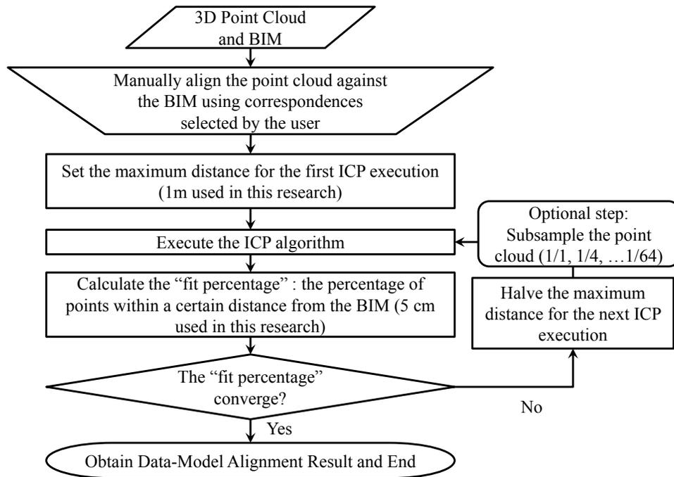
Figure 4 Flowchart of the progressive registration algorithm
