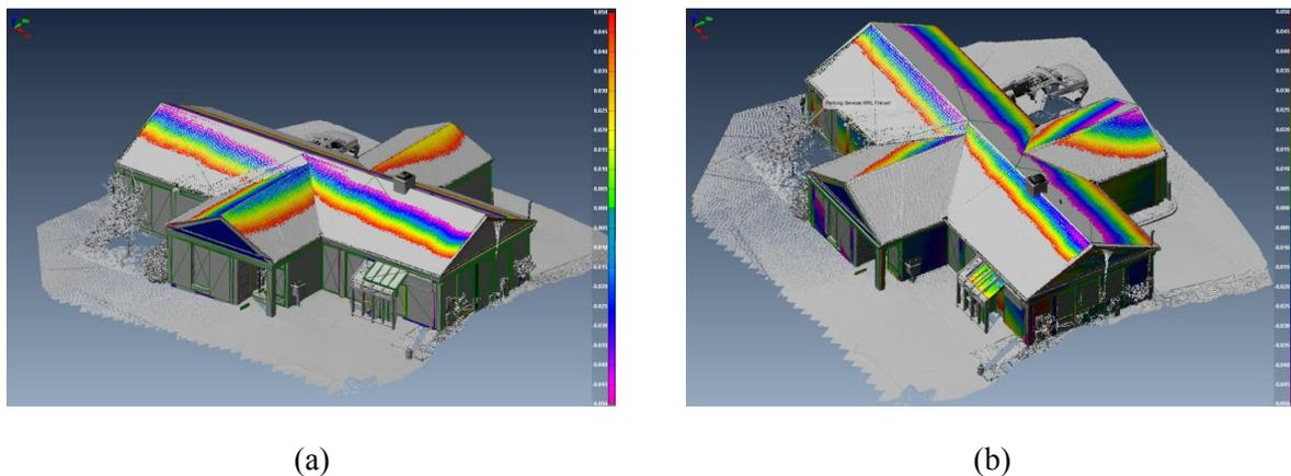
Figure 2 (a) The alignment result of ICP algorithm using a maximum distance of 1m, in which the color scale is from -5 cm (magenta) to +5cm (red), and the points beyond these limits are of the default color, grey; (b) The alignment result of ICP algorithm using a maximum distance of 5 cm.
