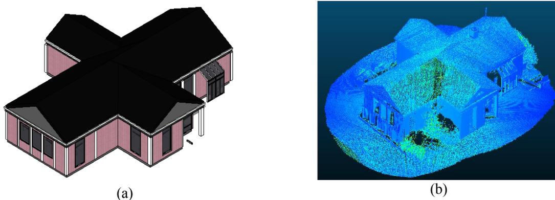
Figure 1 As-is BIM (a) and dense 3D point clouds (b) collected for identifying the as-is BIM modeling errors
