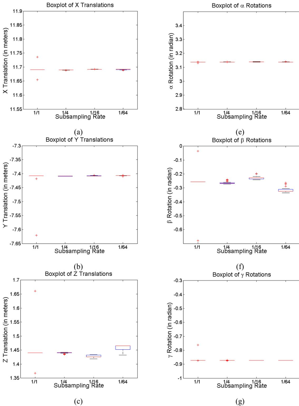
Figure 5 The impacts of subsampling rates on the reliability of the progressive registration results on five different manual data-BIM alignments: each box plot in this figure shows the distribution of 150 registration results (30 repetitions of PRA on each manual alignment × 5 manual alignments).
