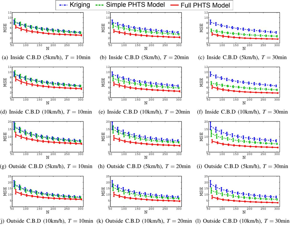
Figure 3: Median Prediction Errors: The horizontal axis denotes the number of full simulations  $N$  and the vertical axis denotes the mean square error(MSE). The vertical bars extend from 25% to 75% quantiles.
