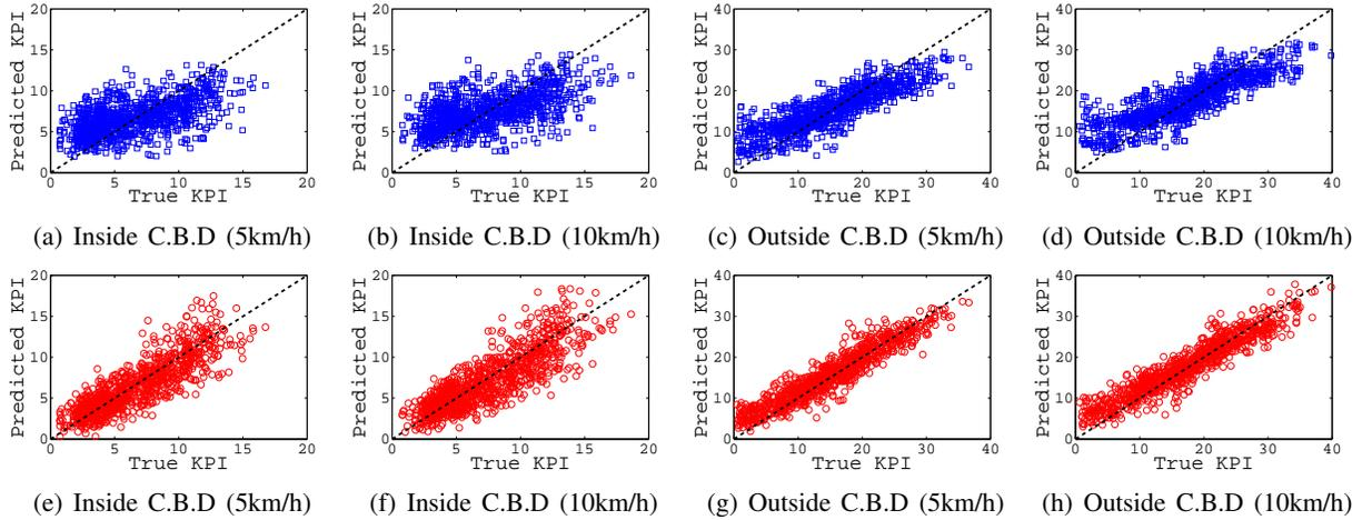
Figure 4: True KPI values and Predicted KPI values when  $N = 60$ : Upper figures (a)–(d) denote results from Kriging while the lower figures (e)–(h) represent results from the full PHTS model at  $T = 30\text{min}$ . The diagonal dashed line denotes the ideal result where the true values and the predicted values coincide.
