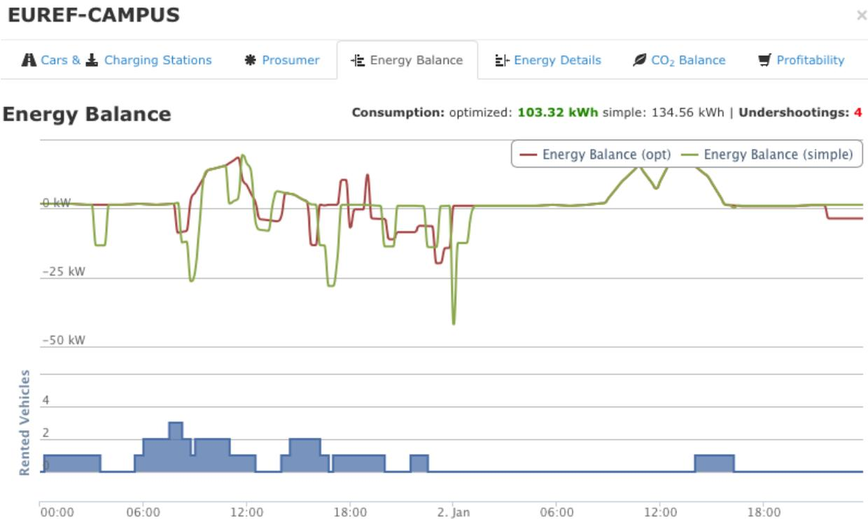
Figure 3: The web front-end comparing the results of intuitive and optimized charging. The tool illustrates the energy balance of both charging profiles (green=intuitive, red=optimized). Furthermore, the absence of electric vehicles is illustrated (blue line at the bottom). It can be seen that returned vehicles correspond with fluctuations in the intuitive energy balance (as a result to the immediate charging process). Absolute consumption values are displayed as well (top right corner).
