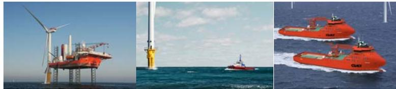
Figure 4: The left image shows a HLV, the middle image show a CTV and the right image show two SOVs.
