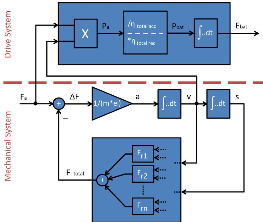
Figure 1: Load model structure.
