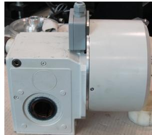
Figure 12: Outer rotor motor and gearbox.
