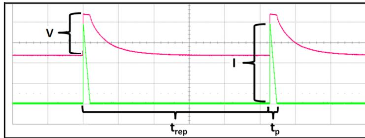
Figure 1: Oscilloscope measurement of  $I$  and  $V$  on different y-axes during a test.
