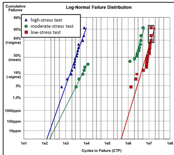
Figure 2: Semiconductor lifetime probability plots from three stress tests.
