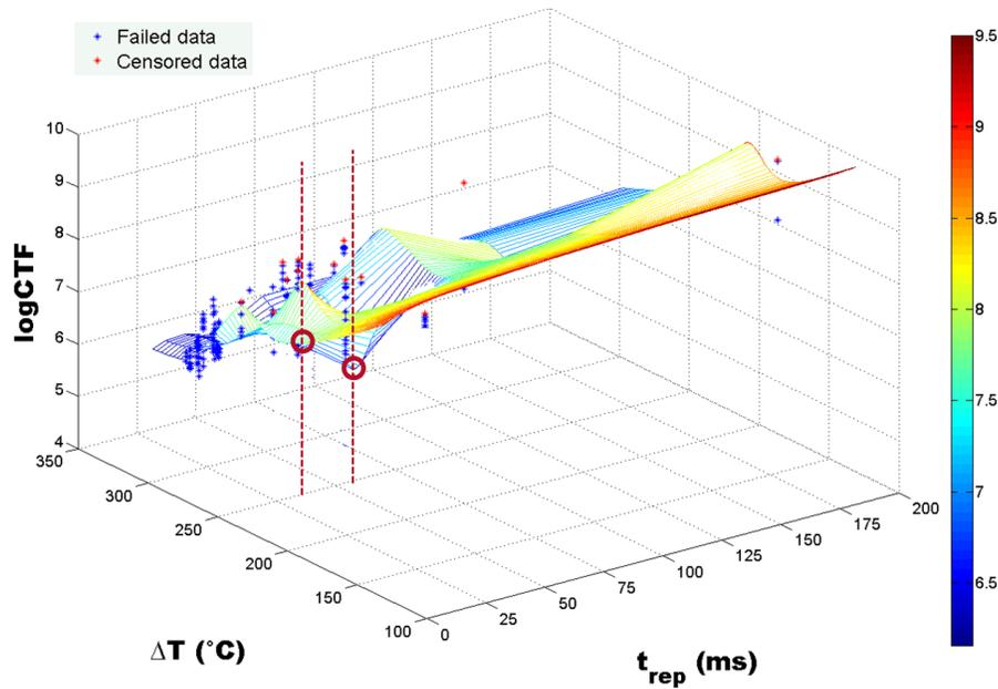
Figure 4: Lifetime prediction for the second mixture component at  $T_{case} = 150^\circ C$  using a standard GP with squared exponential covariance function.
