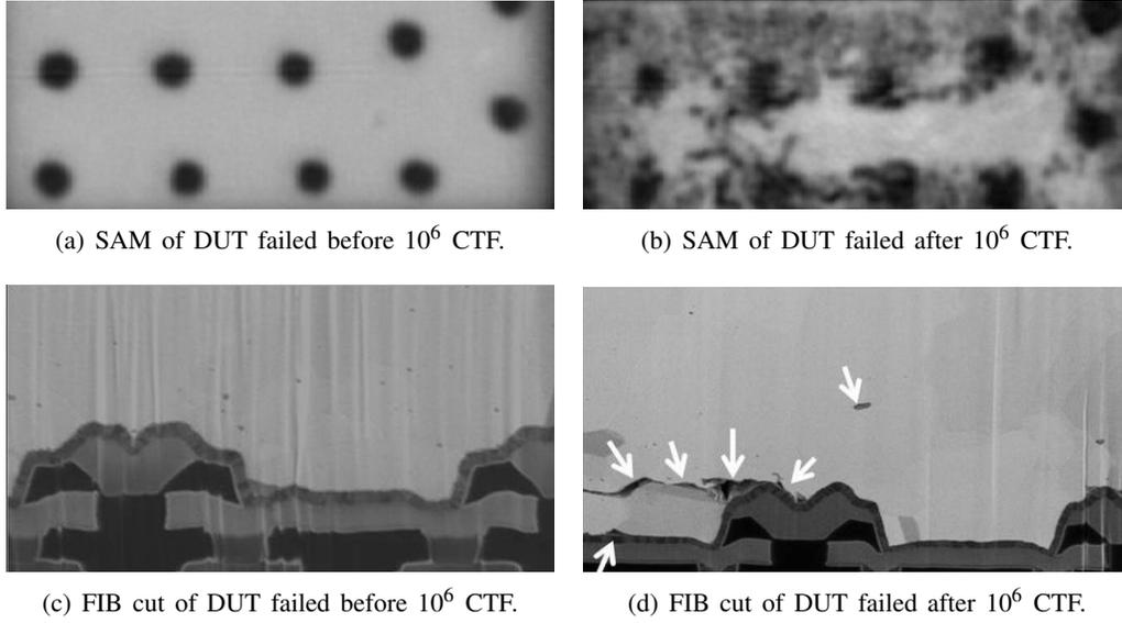
Figure 3: Physical failure inspection reveals different failure mechanisms for DUTs that fail in the first and second mixture component.
