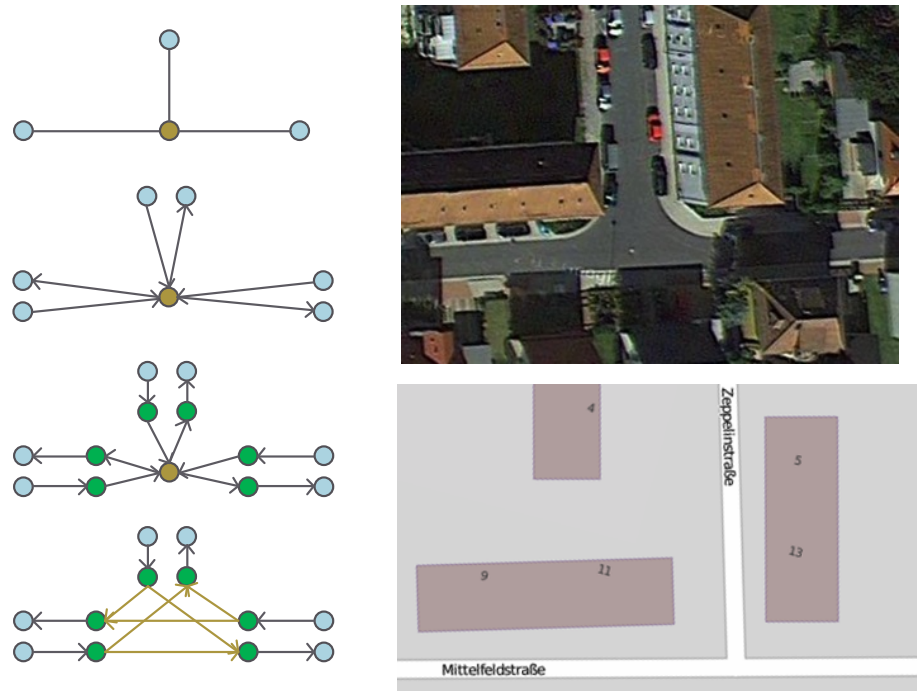
Figure 7: Left side from top to bottom shows the process of creating a more realistic intersection. Lower right side shows a screenshot of the original OSM data and upper left side shows a Google Maps satellite image of the actual intersection.
