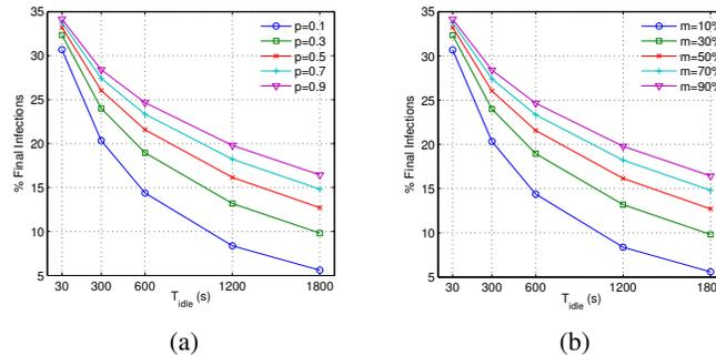
Figure 7: Interaction of  $T_{idle}$  with  $p_{inf}$  and  $m$  for the NRV1 network plotted as a function of the percentages of devices infected at the end of the day (denoted as “% Final Infections”). (a): Shows the interaction between  $T_{idle}$  and  $p_{inf}$  for a low market share ( $m = 10%$ ); (b): Plots the interaction between  $T_{idle}$  and market share,  $m$  for a low probability of infection ( $p_{inf} = 0.1$ ).
