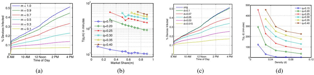
Figure 6: (a): Infection spread with varying market share of the susceptible devices; (b):  $T(q, m)$  for different values of  $q$  and varying market shares of the susceptible devices. Infection spread dynamics with variation in location density ( $d$ ). (c): Infection spread with varying  $d$ ; (d):  $T(q, d)$  changes with varying density of locations.
