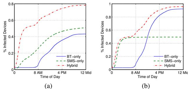
Figure 8: Comparison of the dynamics of Bluetooth, SMS and hybrid malware in the (8a) NRV1 and (8b) NRV2 networks.
