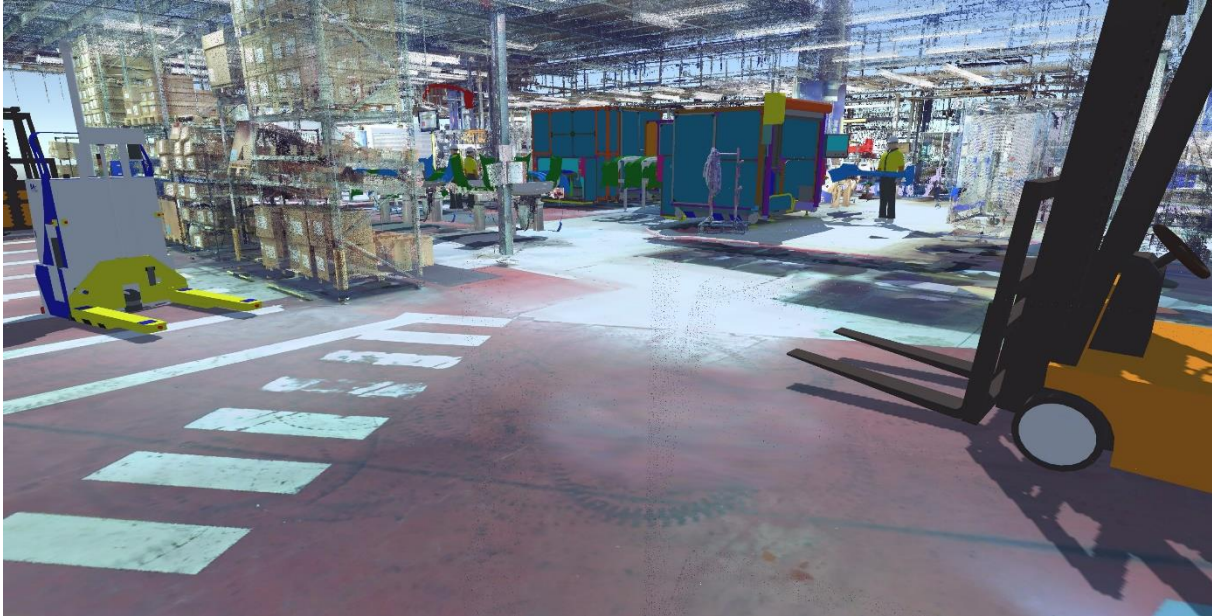
Figure 5: An example of the final model as it would appear when visualized in immersive VR. Forklifts and operators move and perform simulated tasks in the virtual model, consisting of both point cloud and 3D CAD data.
