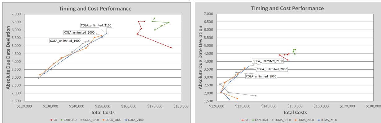
a) Timing and Cost Performance for different parameterized order release models for a loose due date slack. b) Timing and Cost Performance for different parameterized order release models for a tight due date slack.
