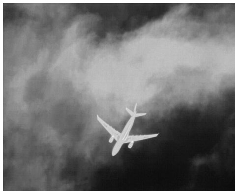
Figure 2. Thermal image of a commercial aircraft captured with the LAADTS thermal sensor.
