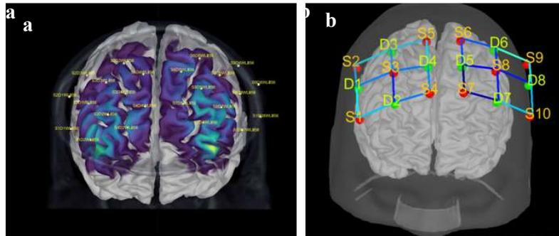
Figure 3. fNIRS channels configuration. (a) Sensitive areas; (b) schematic layout
