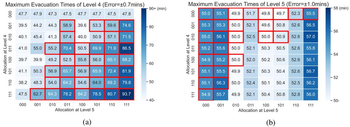
Figure 4: Maximum evacuation times for trolley-ridden patients at Level 4 and Level 5 using different elevator allocations, respectively. The boarded values are the maximum evacuation times for both levels. The overall margins of error with 95% confidence intervals are given.
