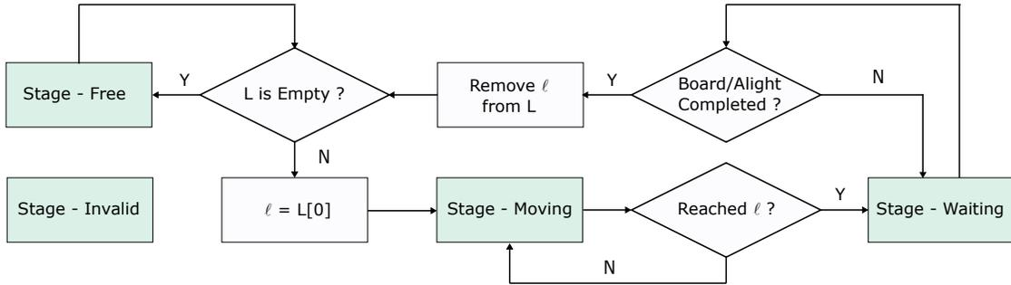
Figure 1: The workflow of an elevator cabin.
