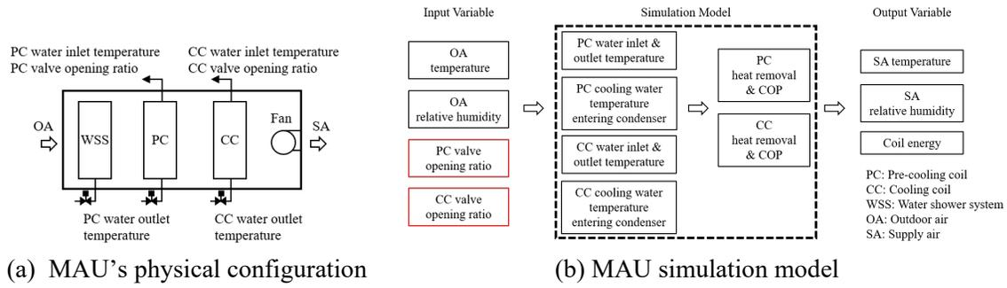
Figure 1: MAU's physical configuration and simulation model (□: Control variable).
