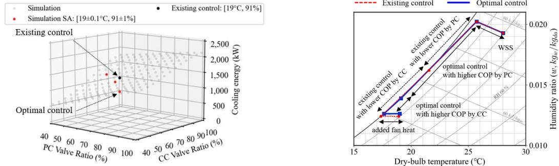
(a) Cooling energy with two valves' opening ratios (b) existing control vs. optimal control
