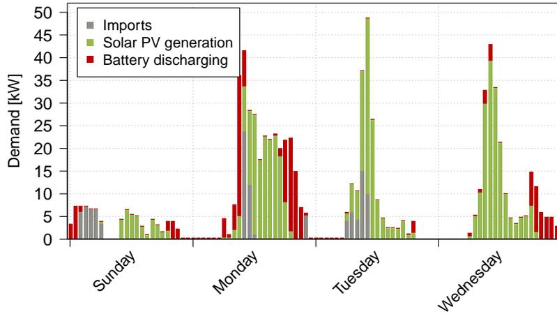
Figure 5: Proportions of EV charging demand supplied by the grid (grey bars), the solar PV system (green), and the BES (red), for an arbitrary 4-day period (the period of July 7 to 10, 2019).
