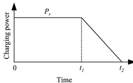
Figure 2: Function approaching the real charging profile.
