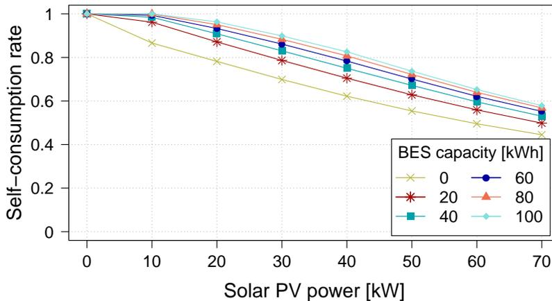
Figure 4: Proportion of self-consumption for the baseline configuration versus installed solar PV power for different BES capacities.
