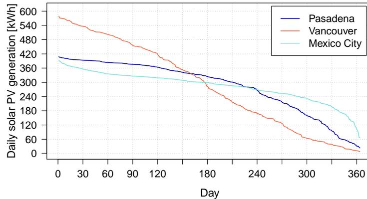
Figure 7: Magnitude-ordered energy generated daily by the solar PV system for a one-year period for the locations Pasadena, Vancouver and Mexico-City.
