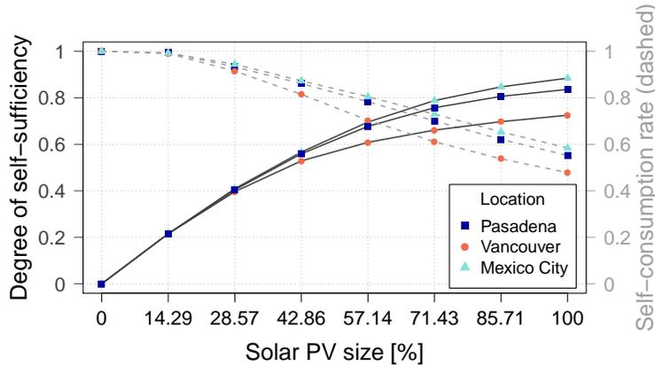
Figure 6: Degree of self-sufficiency (solid lines) and self-consumption rate (dashed lines) for different solar PV system powers for the locations Pasadena, Vancouver, and Mexico-City. Note that the percentage of the solar PV size refers to the respective maximum power value for each location.
