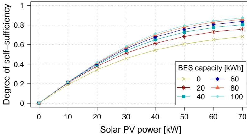
Figure 3: Degree of self-sufficiency for the baseline configuration versus installed solar PV power for different BES capacities.
