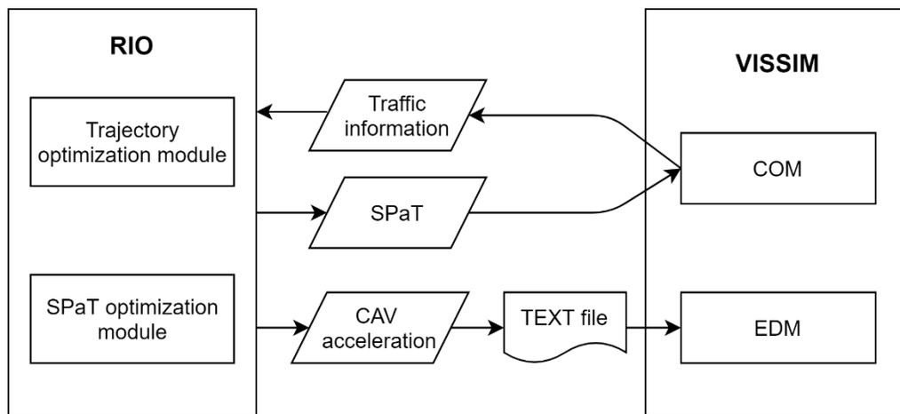
Figure 3. The flowchart of data exchange between VISSIM and RIO.
