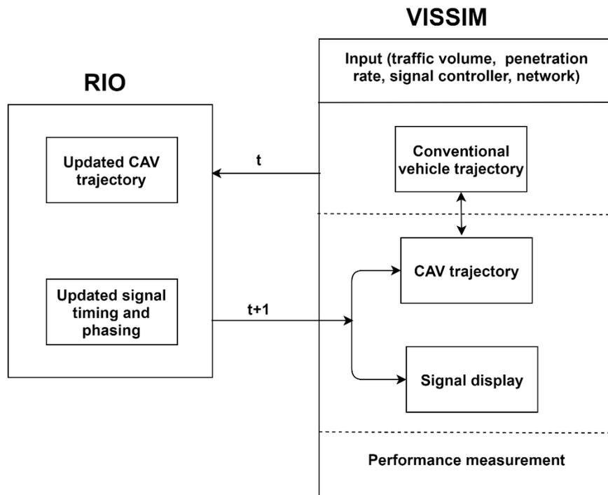
Figure 1. Design of the simulation platform.
