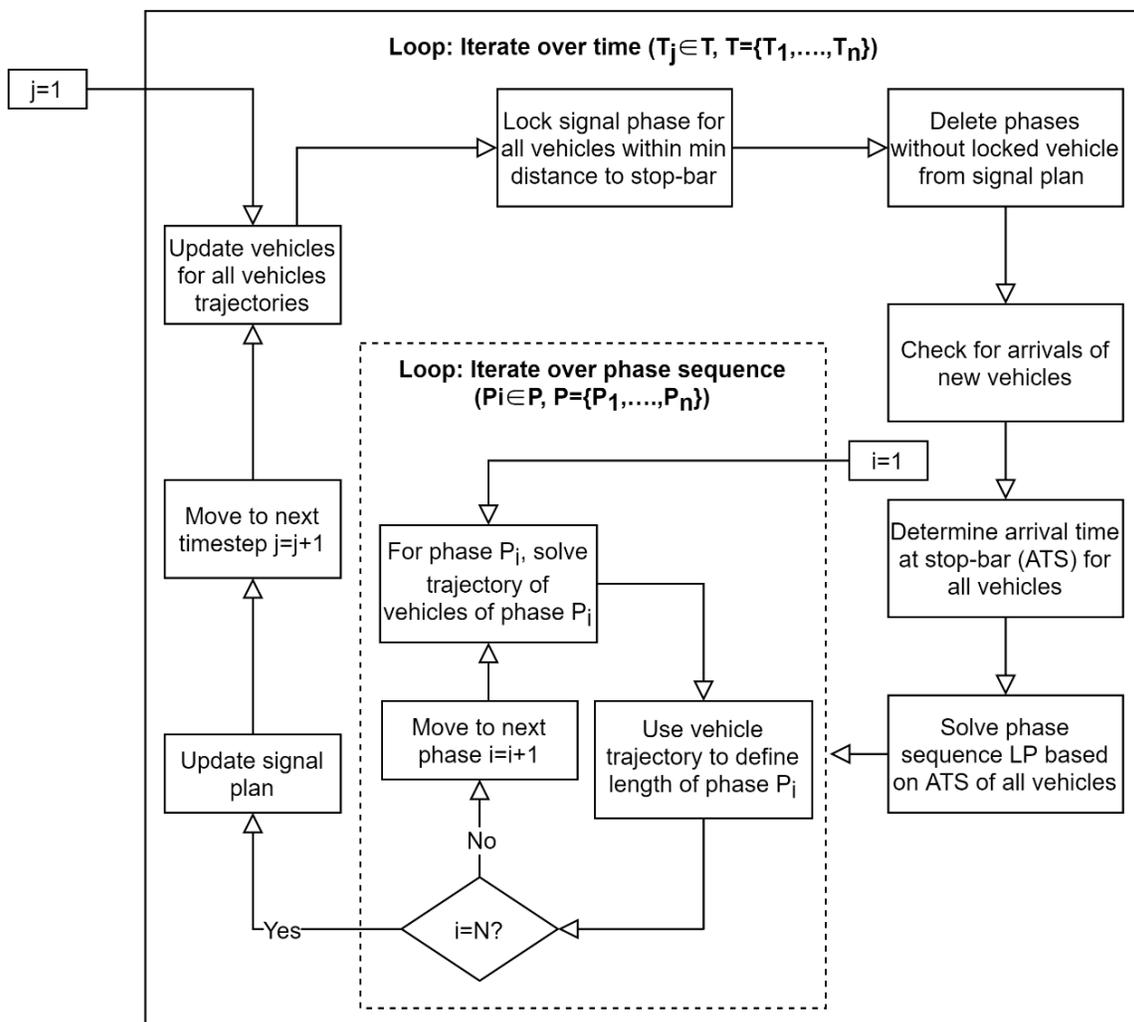
Figure 2. Iteration of the algorithm of joint optimization of signal and trajectory.
