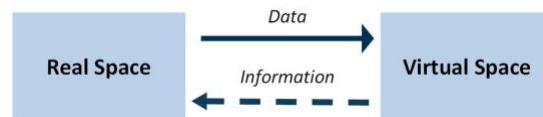
Figure 1: The Digital Twin concept with a real and virtual space with bi-directional flow connecting them (Grieves and Vickers 2016).
