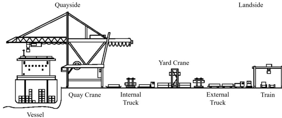
Figure 1: A typical configuration of container terminals modified from Steenken et al. (2004).
